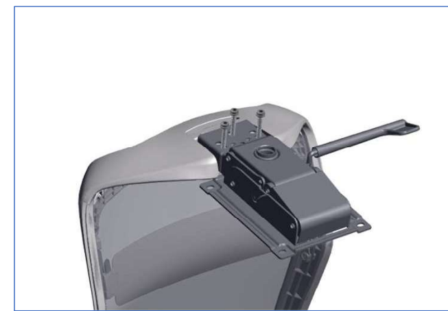
3. Tighten the 3x bolts
