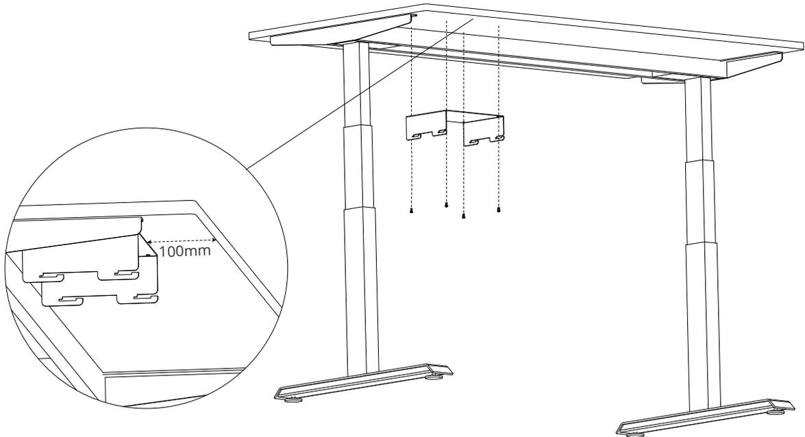
Step 2: Secure Hanging Bracket by screwing in 4 tapping screws.
