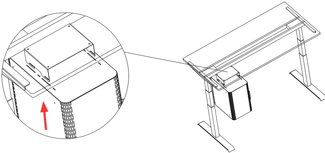
Step 4: Push storage towards the back to allow storage to be securely hooked.
