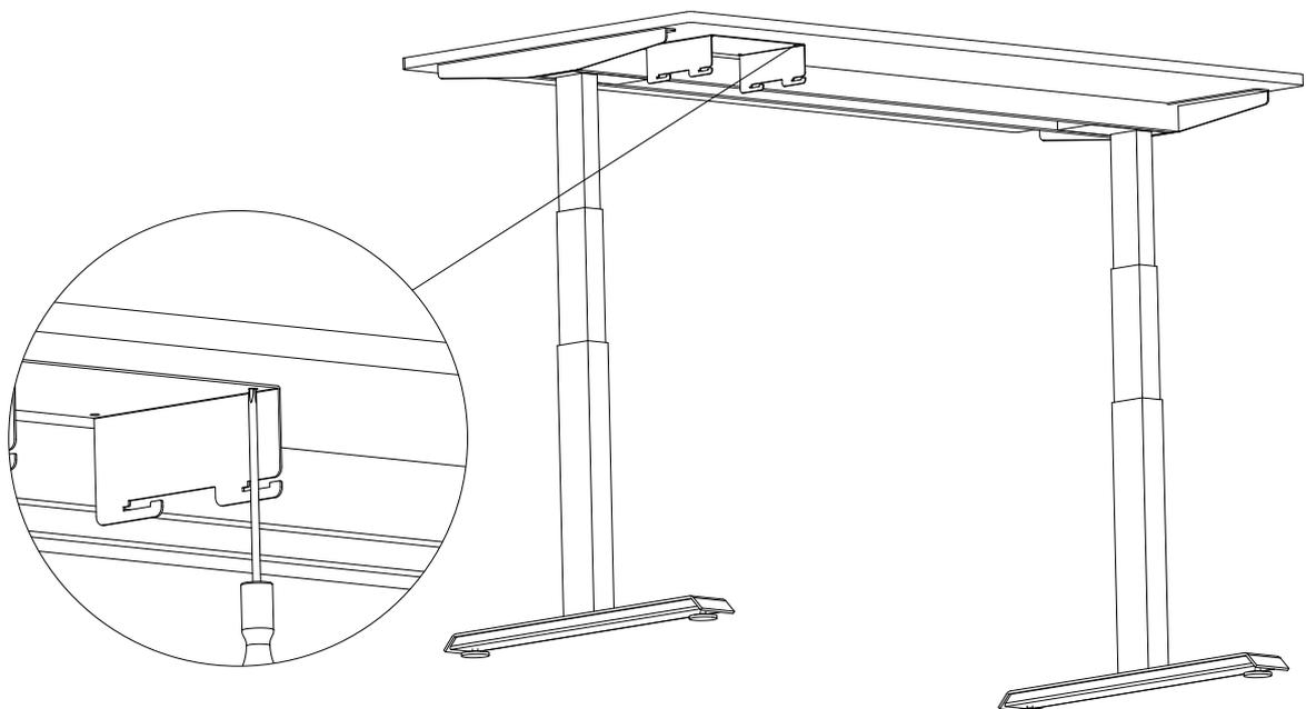
Step 3: Lift storage to Hanging Bracket and insert hook through opening as shown.
