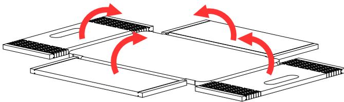
Step 2: Bend each corner and insert H-Bracket to fasten the corners.
