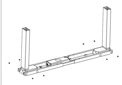
STEP 2: Install the columns on the frames with eight M6\*10 screws
