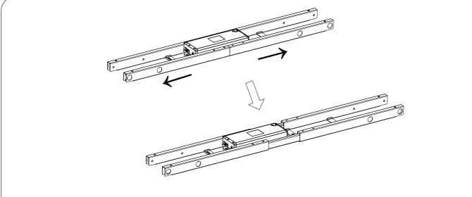
STEP 1: Insert the center rail into the frames, noting the direction of the center rail
