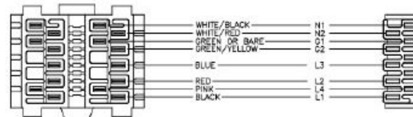
WIRING ORDER 8-WIRE 4-2-2 (3 + 1) DISTRIBUTION END VIEW
