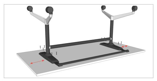
STEP 3: Ensure the frame is located in the centre of the worksurface.
