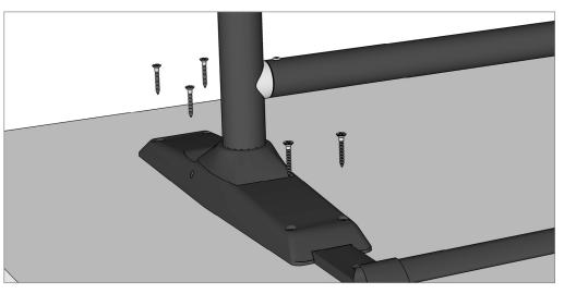
**STEP 4:** Fully tighten all 6 screws on each mechanism.
