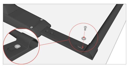
On all tables with width larger than 700mm, secure the pull bar with STEP 5: the supplied washer and screw in the location pictured above (slot end closest to the pull-bar). Leave screw 1 turn from tight so the pull-bar can be operated smoothly.
