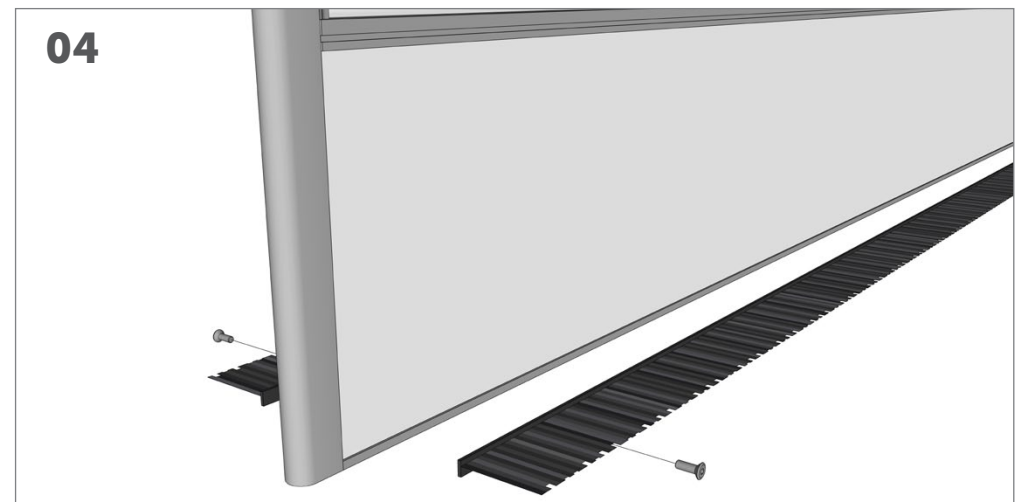
Screw fix the Comseal cable brushes to the base screen. Locate the correct height by resting the black Comseal extrusion against the top lip of the anodised bottom rail of the screen.
