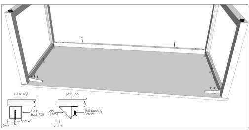
**STEP 2:** Fix desk frame to worktop, allowing for a 5mm overhang on all sides. Fully tighten all rail to frame screws.
