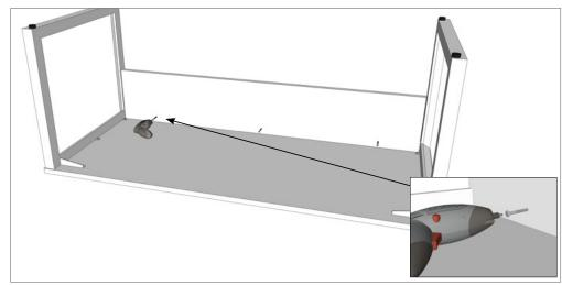
**STEP 4:** Pre-drill holes into the modesty and fully tighten the modesty to the rail with provided screws.
