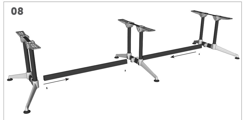
Place all assembled leg sets together using the bottom rails, and fully tighten the M8x16mm bolts to lock all legs together.
