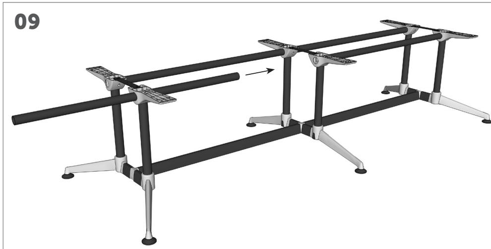
Slide each top rail through the upper wrists, making sure they are located in the centre of the frame.
