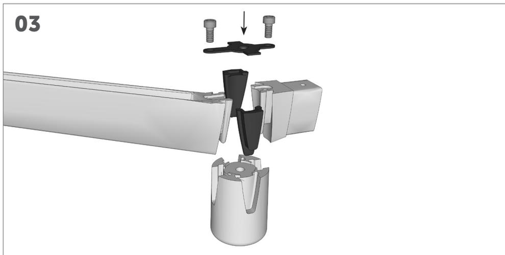
Slide the large foot, T tube connector and 2 cross collar plugs into the collar, place the minus gasket on top, and fully tighten the 2 M8x16mm bolts into the collar. *(Repeat with all cross collars)*
