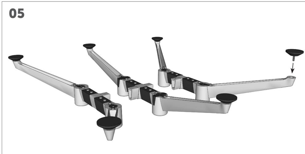
Screw all glides into the base of the large feet, leaving the glides one turn from tight (then they can be adjusted easily if the floor is uneven).
