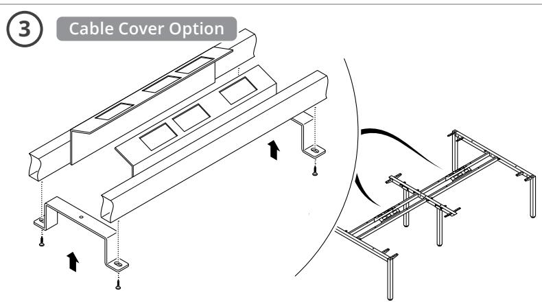
If using our laminate Cable Covers, install the Cable Cover brackets between the facing desks, one on each side of the power/data plate, and one at the end of each frame. Follow the Cable Cover Installation Guide.
