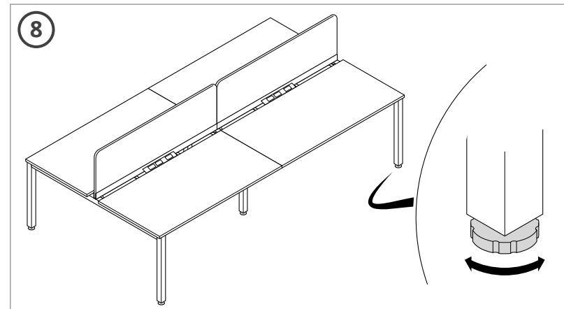
Adjust the feet so the desk pods are level and stable. Fully tighten all rails and frame bolts.
