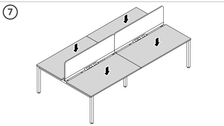
Install the worksurfaces so that they are flush with the back of the frame and/or the power/data plate. Keep the desk overhang equal along the front and sides. If using our laminate Cable Covers, install them now. Follow the Cable Cover Installation Guide.
