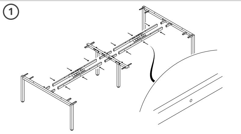
Assemble the frames and rails together. Leave the bolts of the frame loose, one turn from tight. Frame bolts are tightened at step 8. Holes for cable trays on sides of rails must face out to the user.
