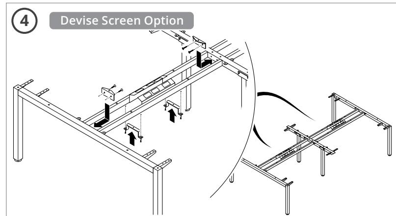
If using our Axis spine screens, install the two end brackets and the two middle supporting brackets between each facing pair of desks. The end brackets fasten to the inside of the leg frame with the single hole facing up. The middle brackets fasten to the threaded holes in the underside of the rail.
