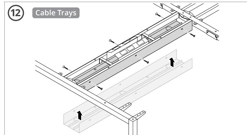
Attach the cable trays to the side of the frame using the bolts provided.
