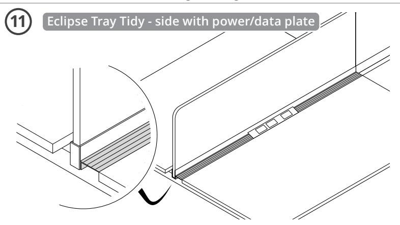
For a side with a power/data plate, use two lengths of Tray Tidy. On each side of the power/data plate, ensure one end of the Tray Tidy is flush with the end of the extrusion, and the other end of the Tray Tidy is behind the power/data plate. Peel the backing tape and stick the Tray Tidy to the extrusion.
