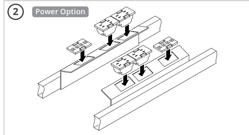
If using our desk power, install the power/data plates, outlets, and wiring. Follow the Electrical Installation Guide provided. Cable trays are installed at step 12.
