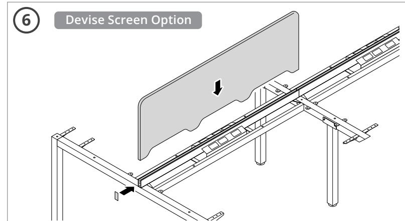
Insert the spine screen fully down into the extrusion, keeping the ends of the screen flush with the end of the extrusion. Take care not to damage the screen while exerting pressure downwards. Fix a spine end cap to each end of the extrusion.
