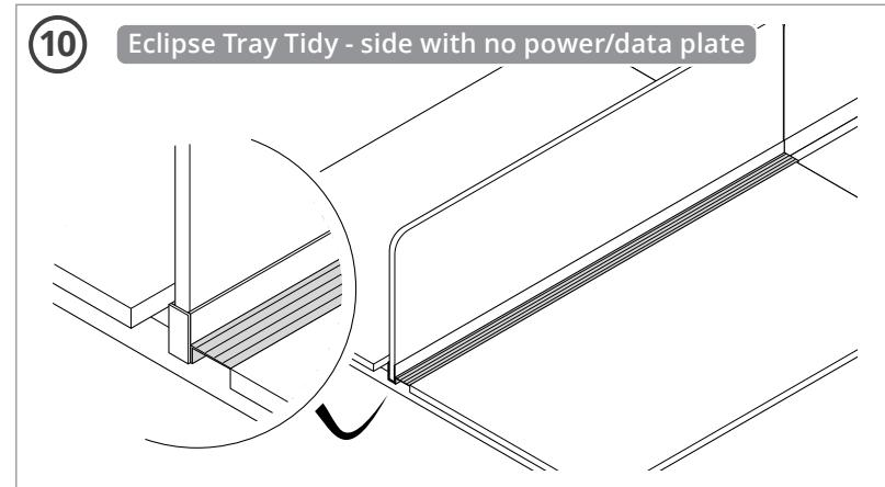
For a side with no power/data plate, use one full length of Tray Tidy. The ends of the Tray Tidy should be flush with each end of the screen extrusion. Peel the backing tape and stick the Tray Tidy to the extrusion.
