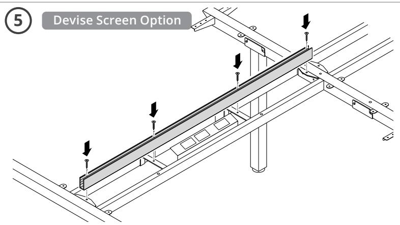
Fasten the screen extrusion to the supporting brackets using the bolts provided. Adjust the screen extrusions along the desks to eliminate gaps between them. Adjust frame to align holes if necessary.
