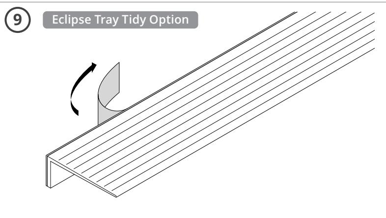
If using our Eclipse Tray Tidy covers, first place the Tray Tidy along the extrusion to check for length and position before exposing the adhesive. The ridged side of the Tray Tidy faces up, with the adhesive side against the extrusion, and the bottom edge resting on the metal frame.
